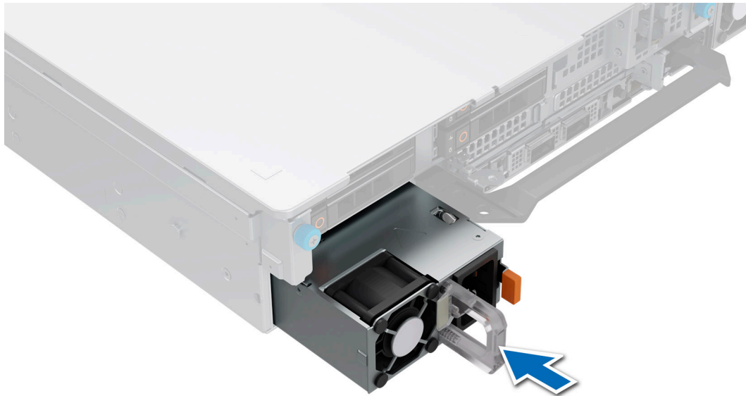
Figure 204. Installing a power supply unit
