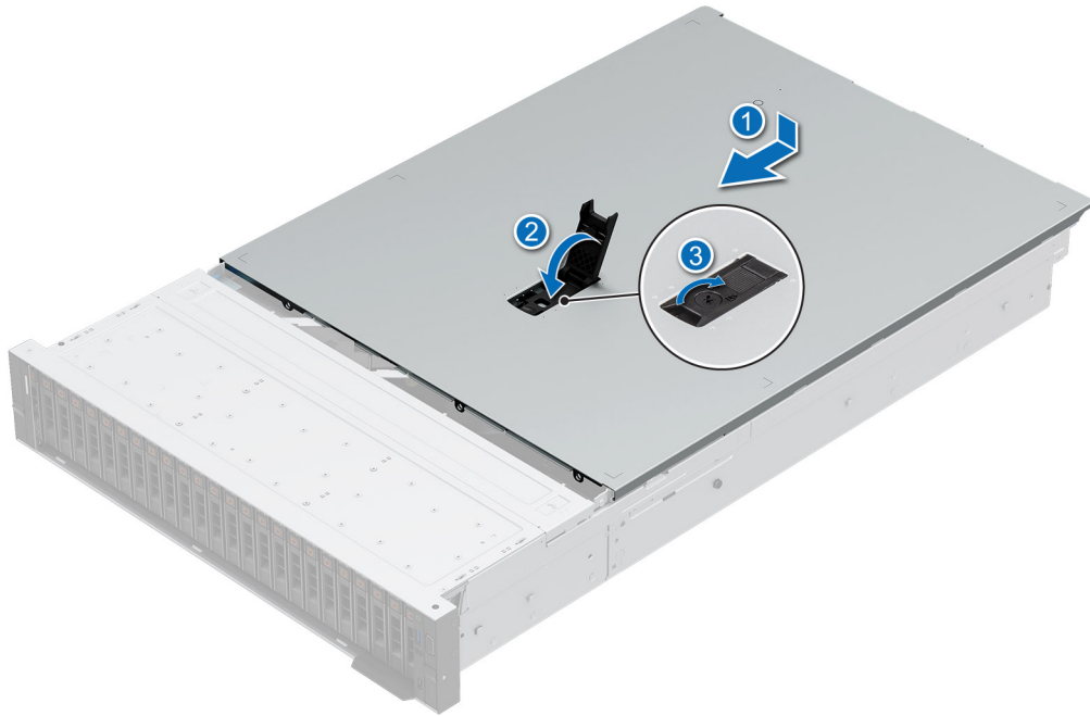
Figure 26. Installing the system cover
